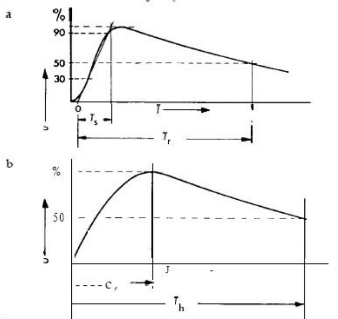
Fig. 4 Standardized test voltages
